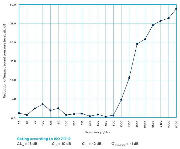
These results are based on a test made with an artificial source under laboratory conditions (engineering Method) with the specified reference floor.
