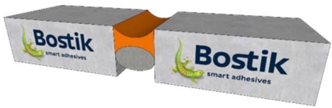
Example 3: Contraction of the building materials due to temperature remittance. Result is that the joint in between of the adjacent building materials will be 'wider'.
