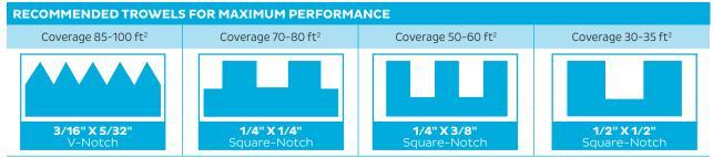
Trowel size is suggested to maximize mortar transfer/coverage. Periodically check coverage during installation. Uneven substrate may require the use of either a leveling/patching material, or larger notched trowel for proper mortar coverage.
