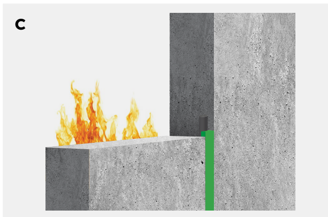
Single sided joint with Bostik FP 401 Fireseal Acrylic in combination with Bostik Backer rod.
