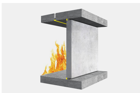
Application example 1: Sealing between stone, wall / floor and wall / ceiling.
