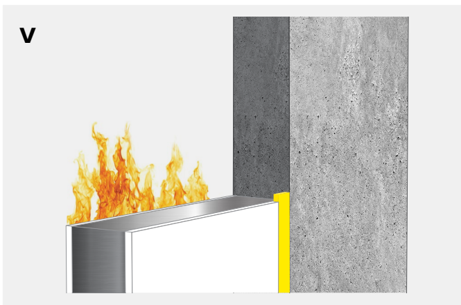
Single sided joint with Bostik FP 403 Fireseal Hybrid .
