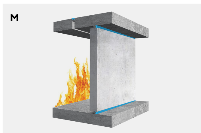
Single sided joint with Bostik FP 402 Fireseal Silicone in combination with Bostik Backer rod.
