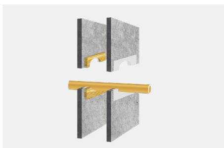
Application example 2: Pipe sealing in drywalls, masonry or concrete walls
