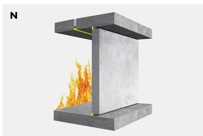
Fire sided single joint with Bostik FP 403 Fireseal Hybrid in combination with Bostik Backer rod.
