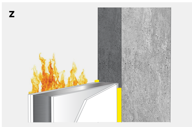
Double sided joint in double plasterboard with Bostik FP 403 Fireseal Hybrid .
