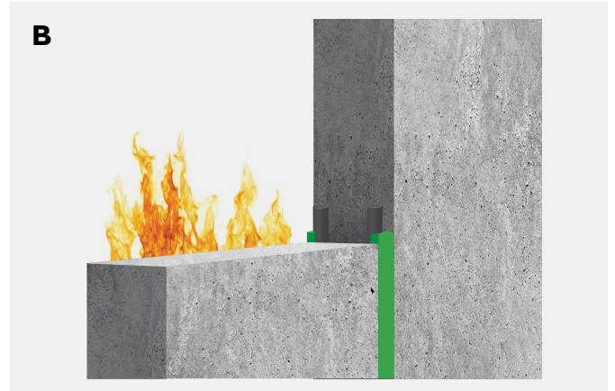
Double sided joint with Bostik FP 401 Fireseal Acrylic in combination with Bostik Backer rod.
