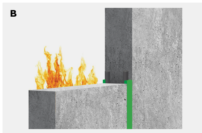
Double sided joint with Bostik FP 401 Fireseal Acrylic in combination with Bostik Backer rod.
