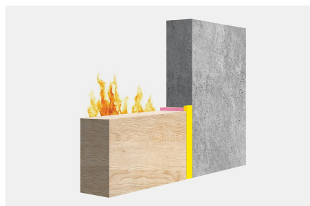
Application example 2: Sealing between stone and wood in combination with FP 403 Fireseal Hybrid.
