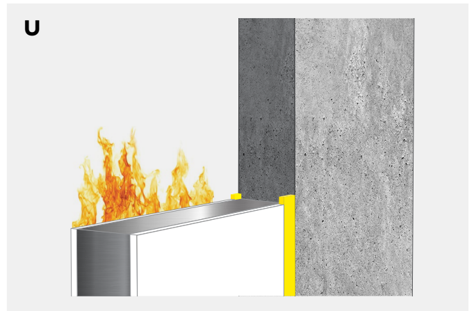
Double sided joint with Bostik FP 403 Fireseal Hybrid .
