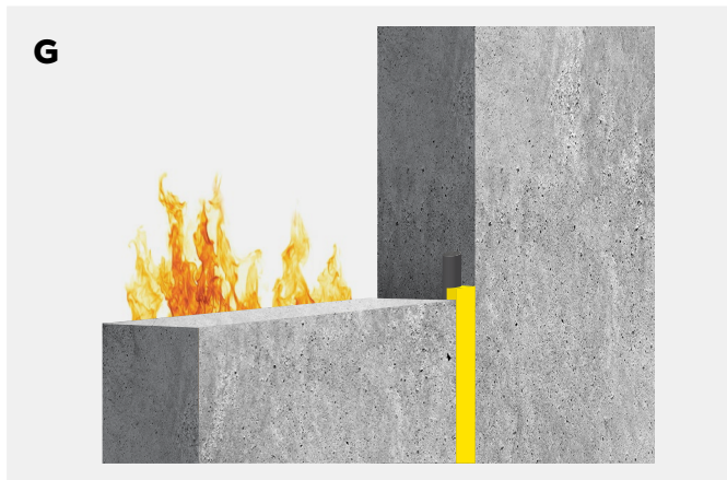
Single sided joint with Bostik FP 403 Fireseal Hybrid in combination with Bostik Backer rod .
