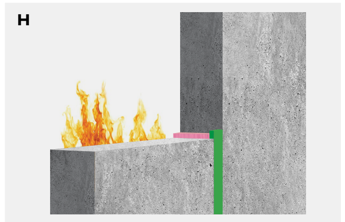
Single sided joint with Bostik FP 401 Fireseal Acrylic in combination with Bostik FP 404 Fire Retardant PU Foam .
