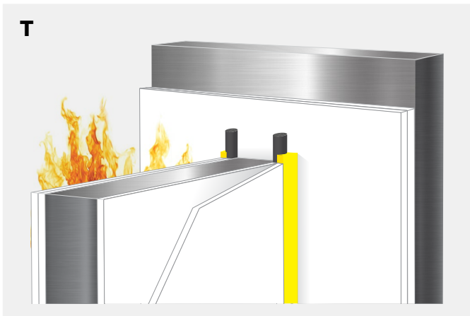
Double sided joint in double plasterboard with Bostik FP 403 Fireseal Hybrid in combination with Bostik Backer rod.
