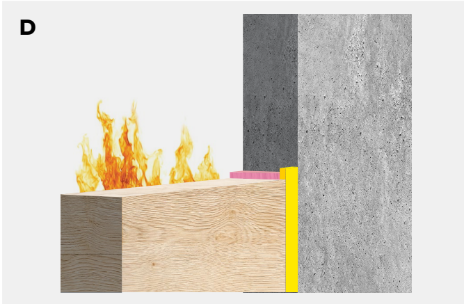
Single sided with Bostik FP 404 Fire Retardant PU Foam in combination with Bostik FP 403 Fireseal Hybrid .
