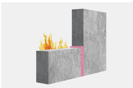
Application example 1: Sealing between stone.
