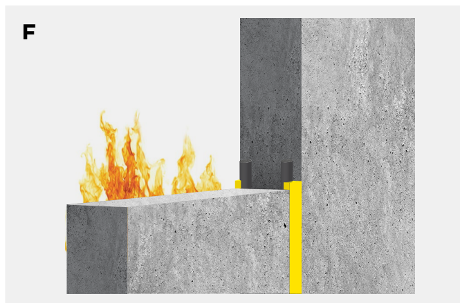
Double sided joint with Bostik FP 403 Fireseal Hybrid in combination with Bostik Backer rod.
