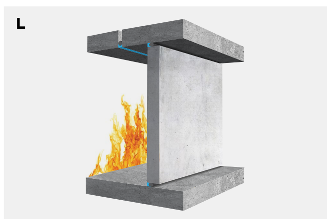
Fire sided single joint with Bostik FP 402 Fireseal Silicone in combination with Bostik Backer rod.
