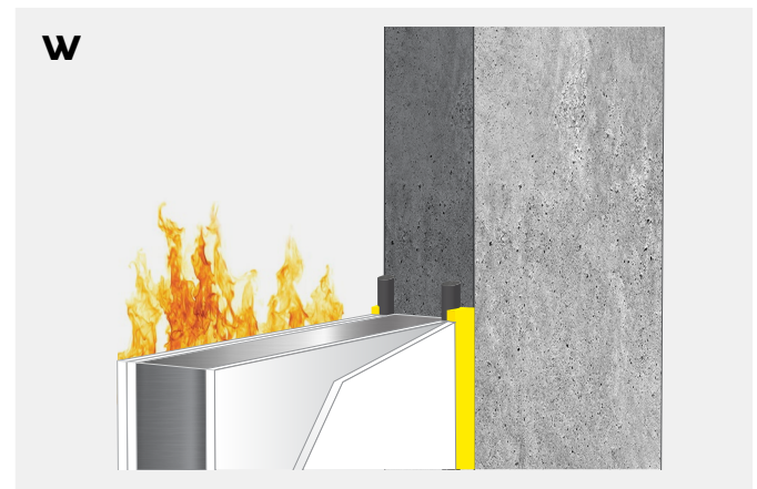
Double sided joint with Bostik FP 403 Fireseal Hybrid in combination with Bostik Backer rod.
