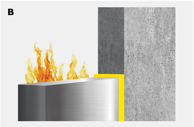
Joint completely filled with Bostik FP 403 Fireseal Hybrid .
