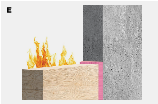
Joint completely filled with Bostik FP 404 Fire Retardant PU Foam .
