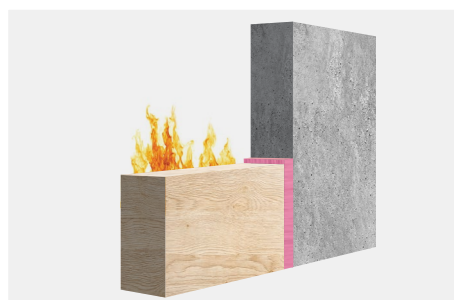
Application example 1: Sealing between stone and wood.
