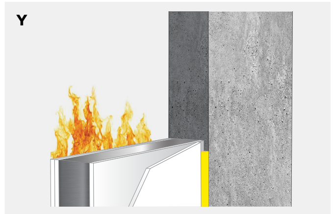
Single sided joint in double plasterboard with Bostik FP 403 Fireseal Hybrid .
