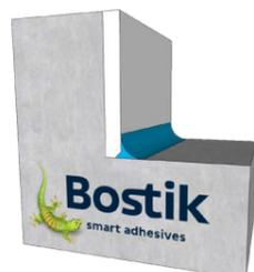
Incorrect applied sealant. The rounded shape of the joint sealant ensures a minimal adhesion to the substrate.
