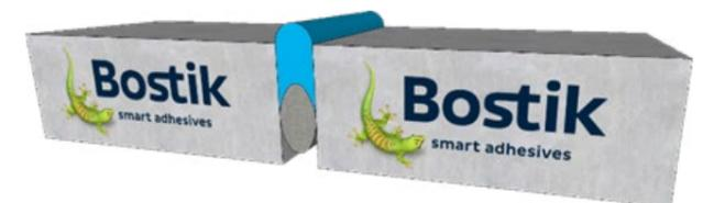
Example 2: Expansion of the building materials due to temperature absorption. Result is that the joint in between the adjacent building materials will be 'smaller'.
