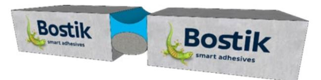
Example 3: Contraction of the building materials due to temperature remittance. Result is that the joint in between of the adjacent building materials will be 'wider'.
