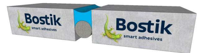
Example 1: Proper applied flexible and elastic joint sealant on a backer rod with the correct installation depth and width.
