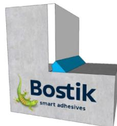
Incorrect applied sealant. The sealant joint is not sufficiently applied and finished, which may cause an adhesion problem.
