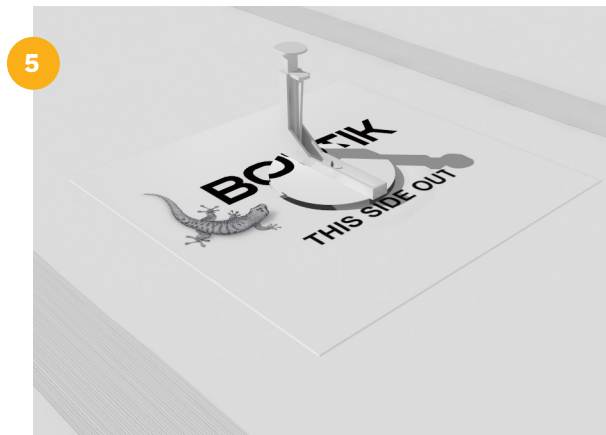
5 Use the specialised tools to cut out the hole for the well.
