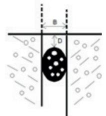
Materials used as backer rods should be weaker that the sealant itself and not obstruct the movement of the sealant, whilst compressing or expanding. Most suitable backer rods are:
