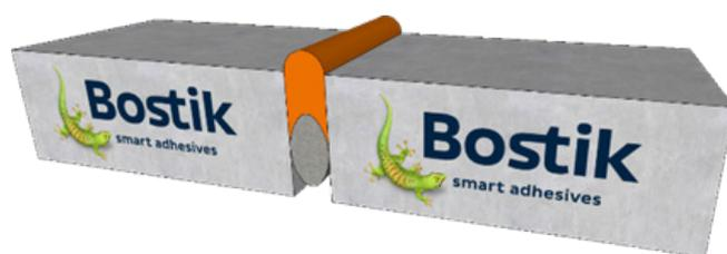
Example 2: Expansion of the building materials due to temperature absorption. Result is that the joint in between the adjacent building materials will be 'smaller'.
