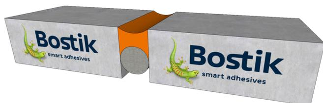
Example 1: Standard correctly applied flexible and elastic joint sealant on a backer rod with the correct installation depth and width.
