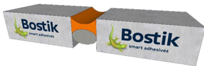
Example 3: Contraction of the building materials due to temperature remittance. Result is that the joint in between of the adjacent building materials will be 'wider'.
