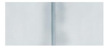
Dark spots or surface discolouration of the paint occurs around the painted joint. Solving this problem can be highly time and material consuming and is therefore costly. Bleeding is a problem that occurs mainly with acrylic caulks, sealants and fillers and is caused by an incompatibility with the paint.
