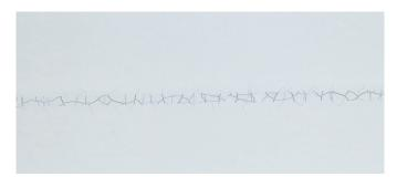
A typical painter's problem is paint cracking. The cause is a distortion of the surface film resulting in long, cracked lines or a pattern of small cracks ("mud" cracking). This is a problem in the finishing process and is difficult to solve afterwards, meaning delay and additional costs.
