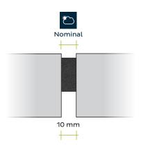
... in the summer period, see the drawing below, the adjacent building elements will elongate due to heat absorption. The joint will compress from 10 till 8 mm. The **BOSTIK M600 TAPE'N'TIGHT BG1** 15/5-10 could still be the preferred dimension to apply, however...
