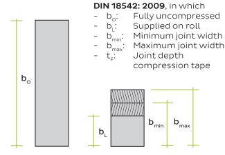
Rule of thumb: b<sub>o</sub>≈5 times b<sub>max</sub>
