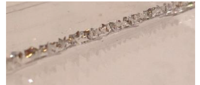
Stress Cracking caused by improper product use
