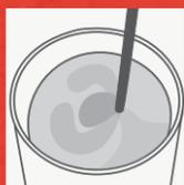
2/ Mix thoroughly with a slow speed electric mixer until a homogeneous mixture is achieved.
