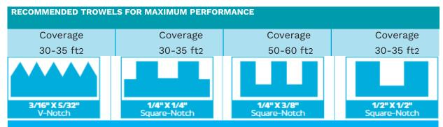
Trowel size is suggested to maximize mortar transfer/coverage. Periodically check coverage during installation. Uneven substrate may require the use of either a leveling/patching material, or larger notched trowel for proper mortar coverage.
