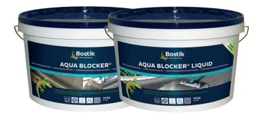
ground water under hydrostatic pressure. Aqua Blocker should not be used to seal parting lines and expansion joints. The joints must be dimensioned and constructed in accordance with the instructions provided. In accordance with DIN 18195, when applied at a weight of approx. 2.3 kg/m<sup>2</sup>, Aqua Blocker achieves crack-bridging performance of > 5 mm with a cured coating thickness of 1.5 mm.
