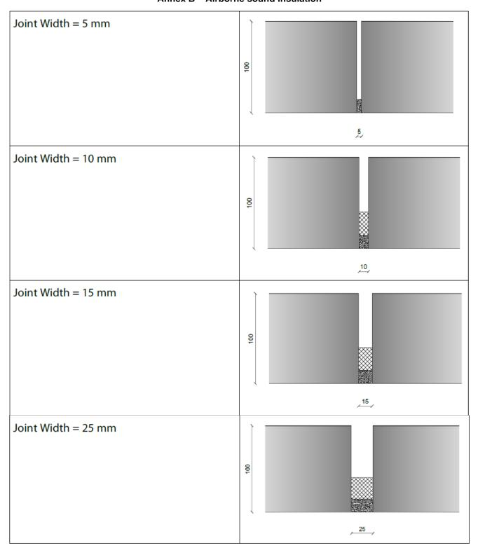
The Bostik FP 401 Fireseal Acrylic sealant, 10 mm depth is backed with PU / PE backer rod.
