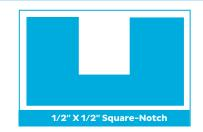
Trowel size is suggested to maximize transfer/coverage of mortar. Periodically check coverage during installation.
