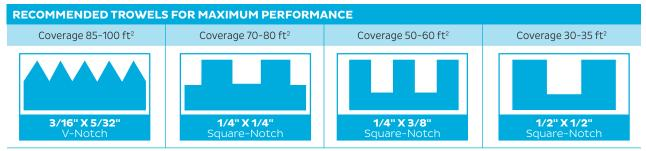
Trowel size is suggested to maximize mortar transfer/coverage. Periodically check coverage during installation. Uneven substrate may require the use of either a leveling/patching material, or larger notched trowel for proper mortar coverage.
