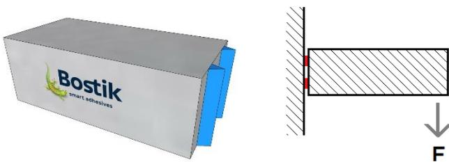
The equation we need to use is: ' $m = F \times L$ '. The force (F) and the length (L) are two factors we know, so the sum will be ' $m = 49,03 \text{ (N)} \times (1000/250\text{mm})$ '. The mass of the so called free hanging part of the concrete block equals 196,12 N/20 kg.
