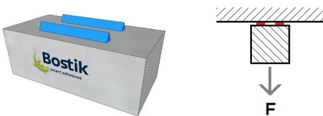
The mass of the block is 5 kg. The gravity acting on the block is 9,81 m/s, meaning that the force 'F' ( $F = m \cdot a \Leftrightarrow 5 \times 9,81$ ) equals 49,03 N/5 kg.
