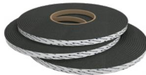
FoamTape™ is part of the complete PanelTack™ system and serves as a spacer for the adhesive bead, to ensure the proper adhesive thickness between the panel and the support structure. FoamTape™ provides an initial fixation of the panel or substrate until the PanelTack HM™ adhesive has cured, while ensuring a strong, lasting bond.
