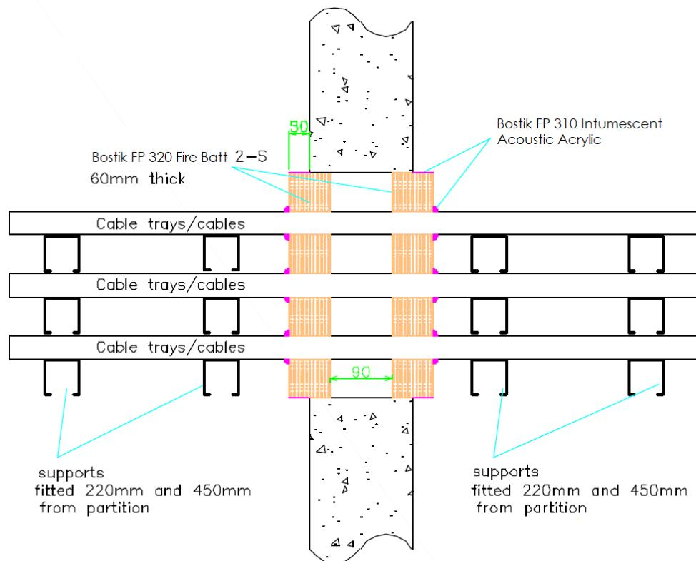
**A.1.6.1 Two side penetration seal with cables**
