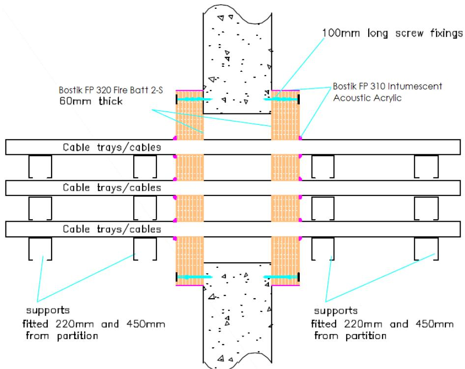
**A.1.7.1 Two side penetration seal with cables**
