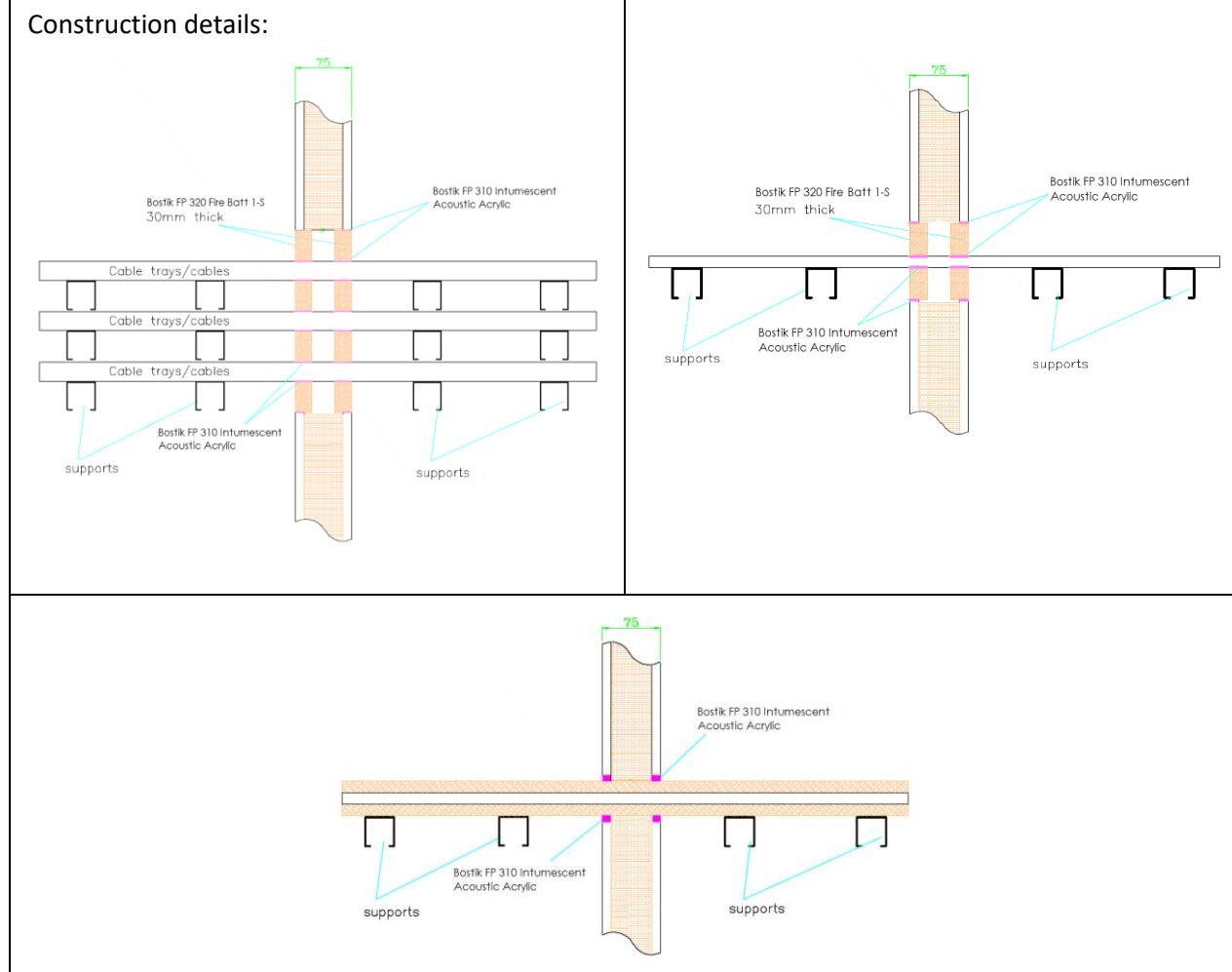
**A.3.1.1 Double side penetration seal with cables**
