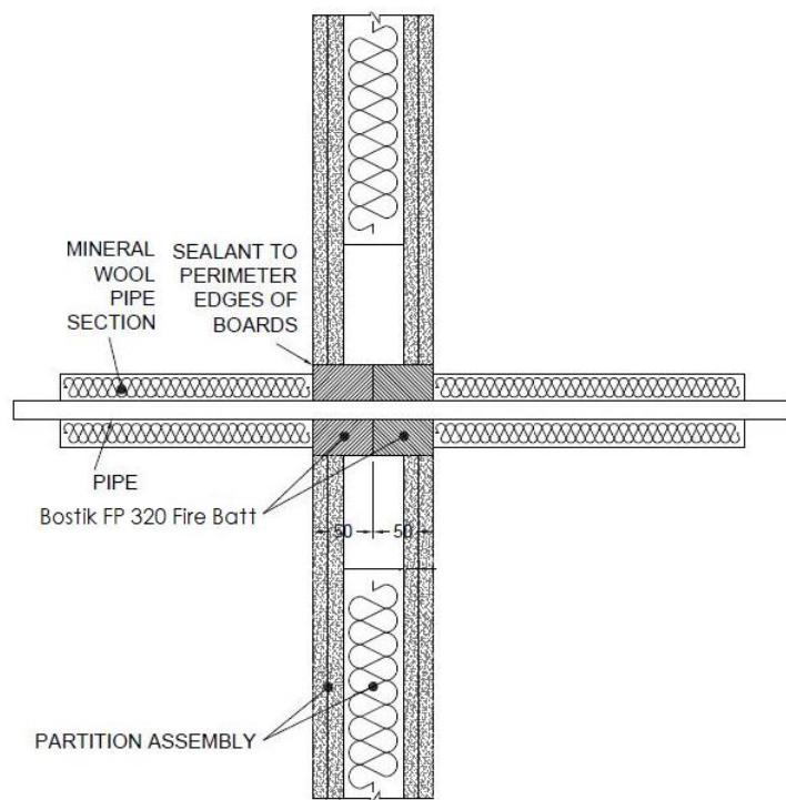
\* Minimum 600 mm long insulation required for Alupex pipe.
